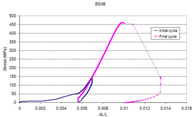
Fig. 8 Average stress versus average shortening curve of BS4B panel
