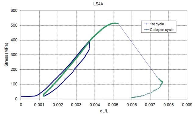
Fig. 10 Average stress versus average shortening curve of LS4A panel
