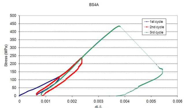
**Fig. 7** Average stress versus average shortening curve of BS4A panel
