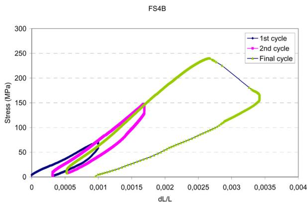
**Fig. 5** Average stress versus average shortening curve of FS4B panel
