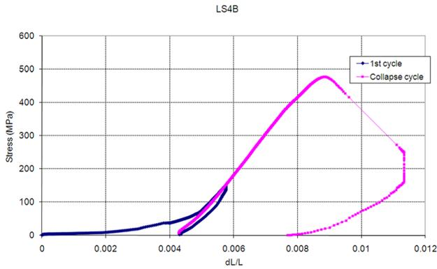
Fig. 12 Average stress versus average shortening curve of LS4B panel
