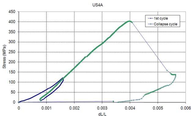
Fig. 13 Average stress versus average shortening curve of US4A panel
