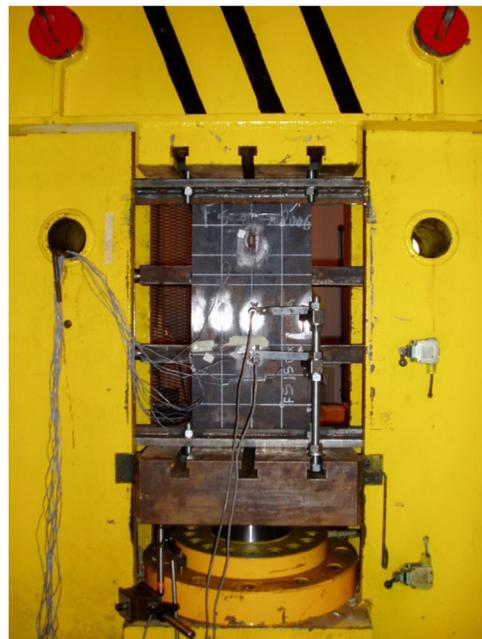
Fig. 3 Setup of the 200 series test of stiffened plates
