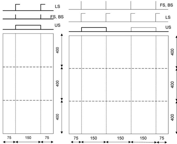
**Fig. 1 Geometry of stiffened panels for fully S690 steel (FS), mild steel bar stiffeners (BS), and L and U mild steel stiffeners for narrow and wide panels**
