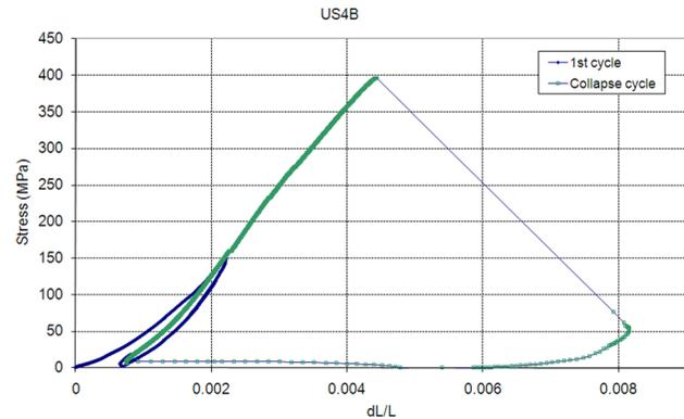
Fig. 14 Average stress versus average shortening curve of US4B panel
