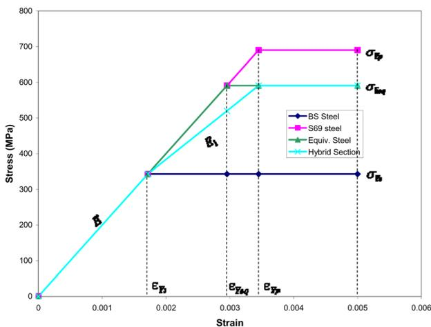
Fig. 2 Material behavior of mild, S690 steel and equivalent material of hybrid BS specimens
