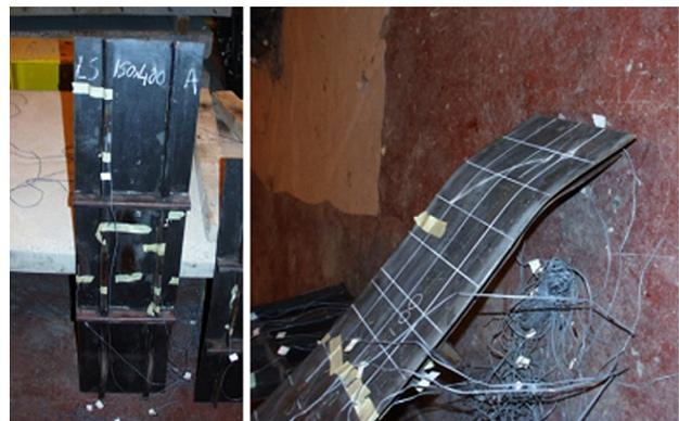
Fig. 11 LS4A panel after collapse
