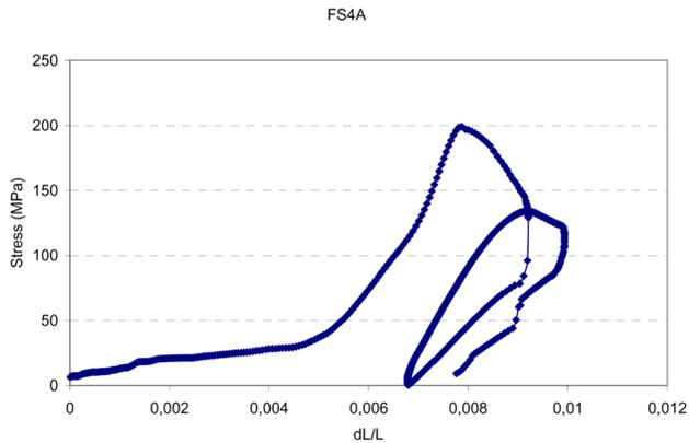
**Fig. 4** Average stress versus average shortening curve of FS4A panel
