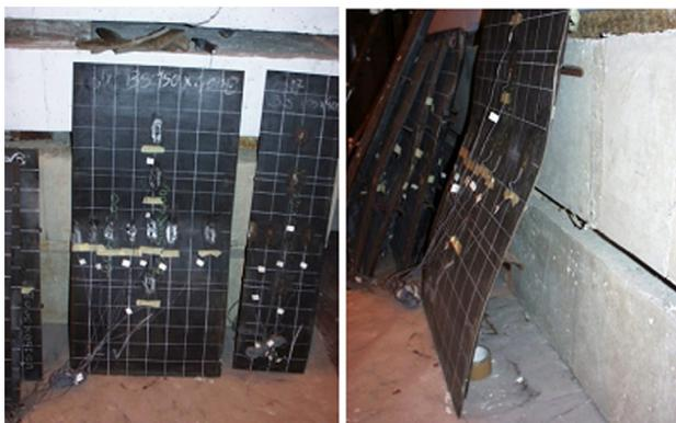
Fig. 9 BS series panels after collapse; detail of residual deformations on BS4B at right
