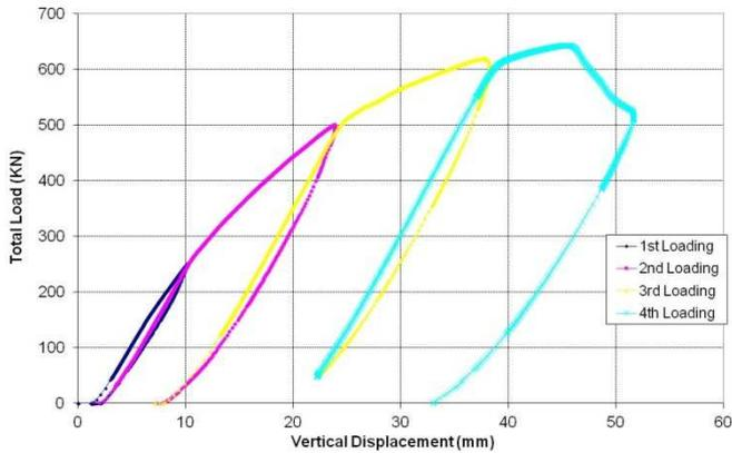
**Figure 4. Vertical load versus vertical displacement on N200 test**
