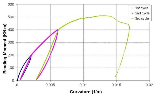
Figure 11. Moment curvature relationship of N300 specimen
