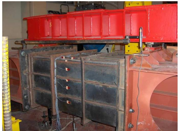
**Figure 6 Setup of one of displacement transducers for measuring the rotation over top panel (N400)**
