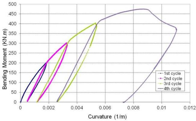
Figure 15. Moment curvature relationship of N400 specimen
