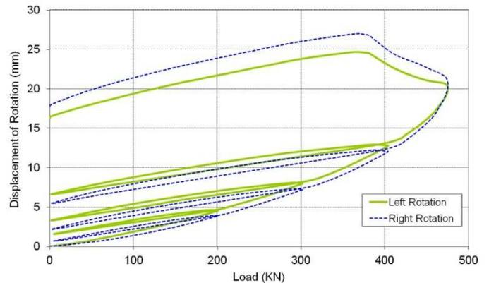
Figure 14- Measurements on the displacement transducers for N400.
