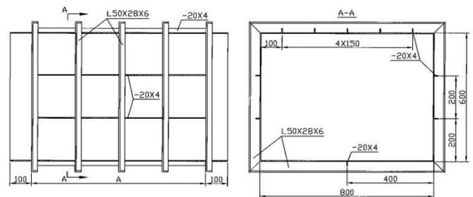
Figure 3. Geometry of the box girder N200.
