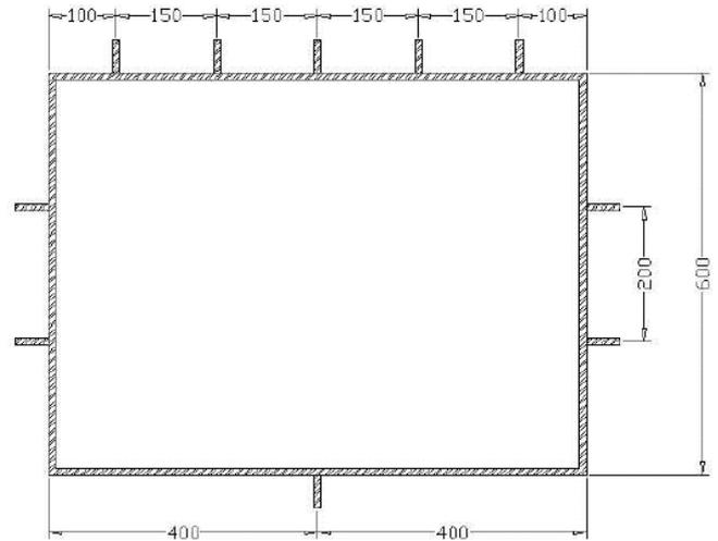
Figure 2. Cross section of the box girders.
