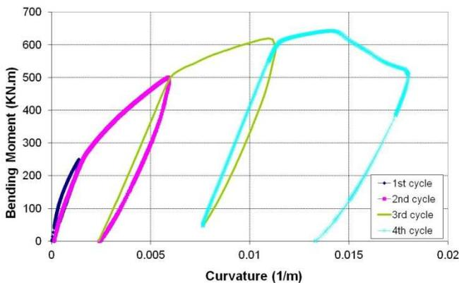
Figure 7. Moment curvature relationship of N200 specimen
