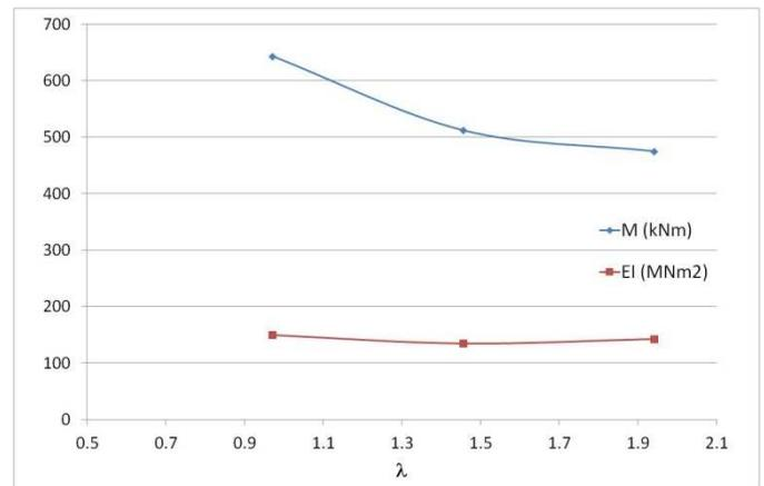
Figure 17 Ultimate bending moment and structural modulus versus column slenderness of top panel
