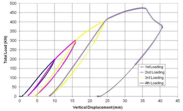
Figure 13 - Vertical load versus vertical displacement on N400 test
