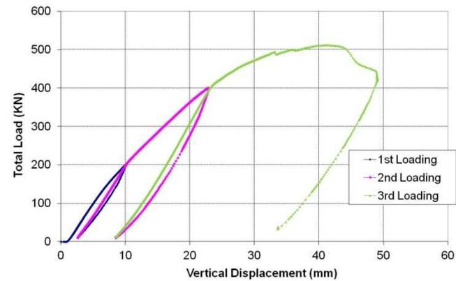
Figure 9 - Vertical load versus vertical displacement on N300 test
