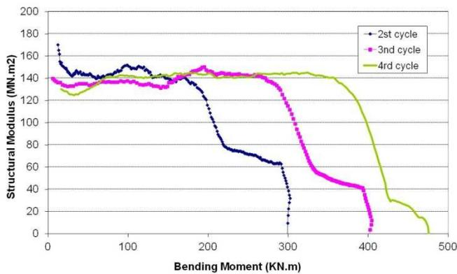
Figure 16 - Structural modulus during loading path for different cycles (N400)
