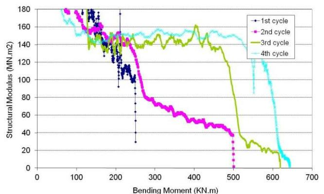
Figure 8. Structural modulus during loading path for different cycles
