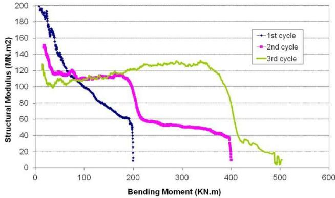
Figure 12. Structural modulus during loading path for different cycles (N300)
