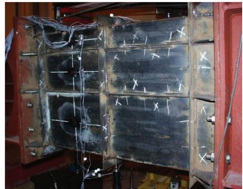
Figure 3. Side panel of box girder M3-100. Details of welding of stiffeners and locations of side strain gauges.
