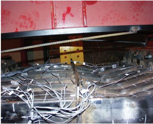
Figure 16. Global residual deformations on top panel.
