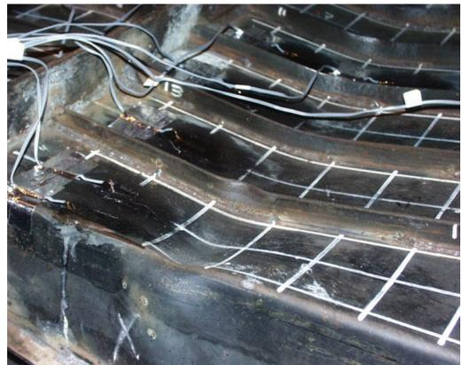
Figure 15. Collapse of box girder in the right bay.
