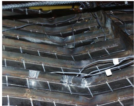
Figure 14. Stiffener's inducer failure in top panel.
