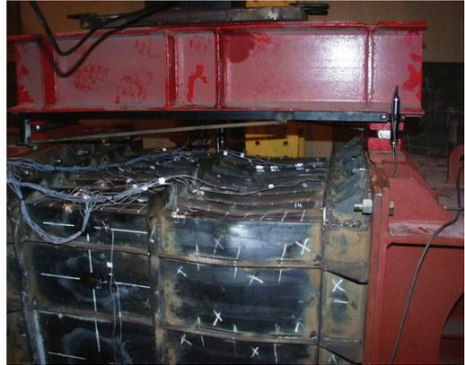
Figure 12. Side panel deformations immediately before collapse (up) and after collapse (down).
