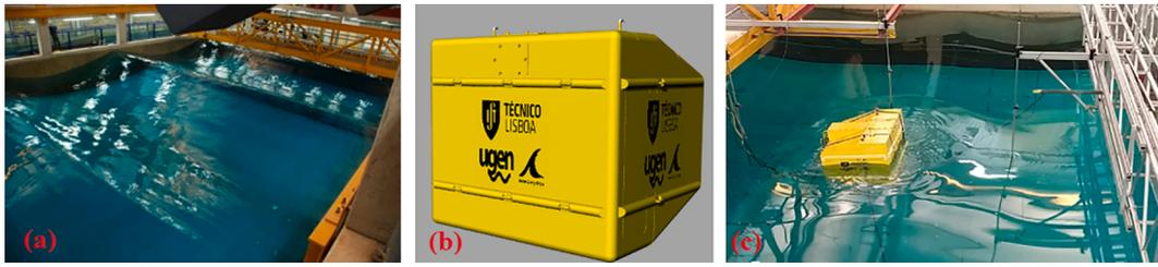
Fig. 3. (a) General view of the ocean wave basin facility; (b) 3D CAD view of the 1:24th-scaled model of the UGEN WEC; and (c) View of the 1:24th-scaled model of the UGEN WEC and the wave gauges during tests at UoP COAST Ocean Basin, Plymouth, UK.
